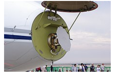
Global Express Weather radar with radome up
