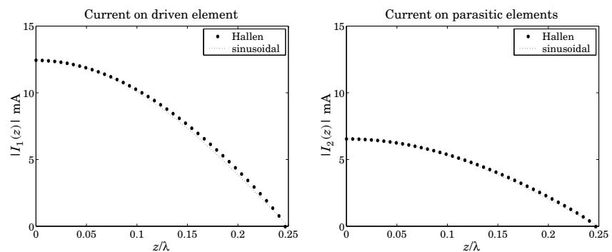
Fig. 25.7.1 Currents on driven and parasitic antennas.
