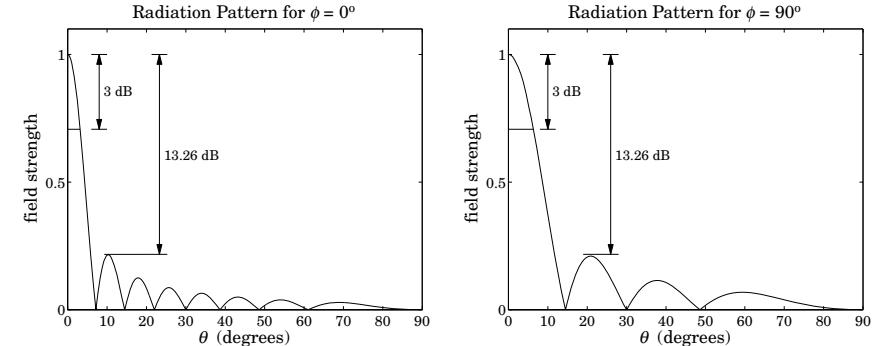
Fig. 18.8.2 Radiation patterns along the two principal planes ( $a = 8\lambda$ ,  $b = 4\lambda$ ).
