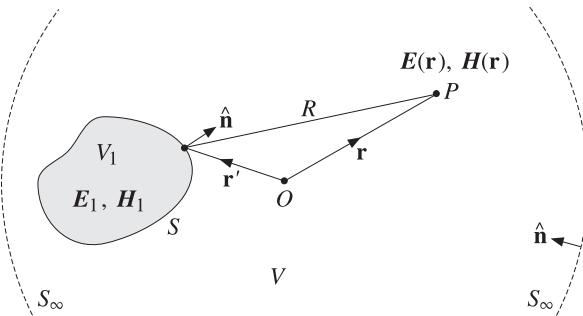
Fig. 18.10.1 Fields outside a closed surface  $S$ .
