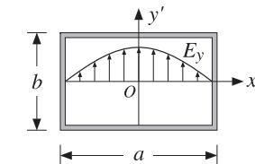
Fig. 21.1.1 Electric field over a waveguide aperture.
