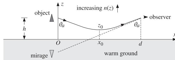
Fig. 7.15.4 Mirage due to a temperature gradient.
