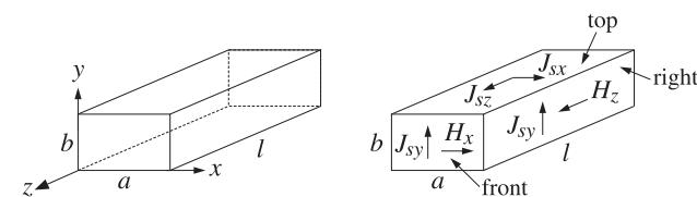
Fig. 9.10.1 Rectangular cavity resonator (and induced wall currents for the TE<sub>n0p</sub> mode.)
