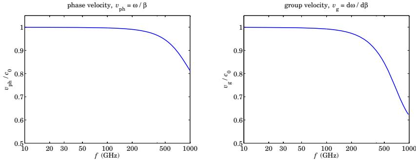
Fig. 10.19.4 Phase and group velocities in units of  $c_0$ .
