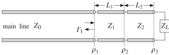
Fig. 13.7.1 Two-section series impedance transformer.
