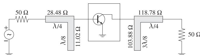
Fig. 14.8.5 Quarter-wavelength matching networks with  $\lambda/8$ -stubs.
