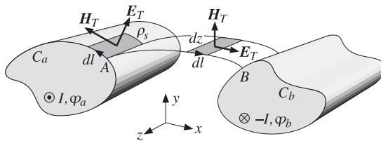
Fig. 11.1.2 Surface charge and magnetic flux linkage.
