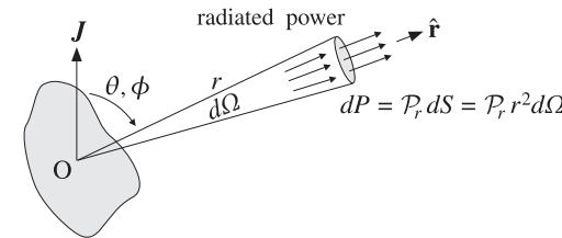
Fig. 15.9.1 Power radiated into solid angle  $d\Omega$ .
