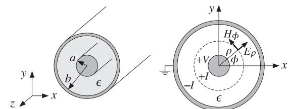
Fig. 11.4.1 Coaxial transmission line.
