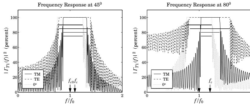
Fig. 8.8.5 TM and TE reflectances for  $n_H = 3, n_L = 1.38$ .
