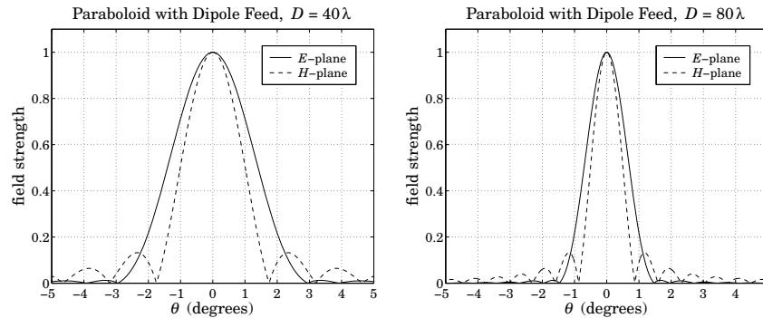
Fig. 21.10.1 Parabolic reflector patterns with dipole feed.
