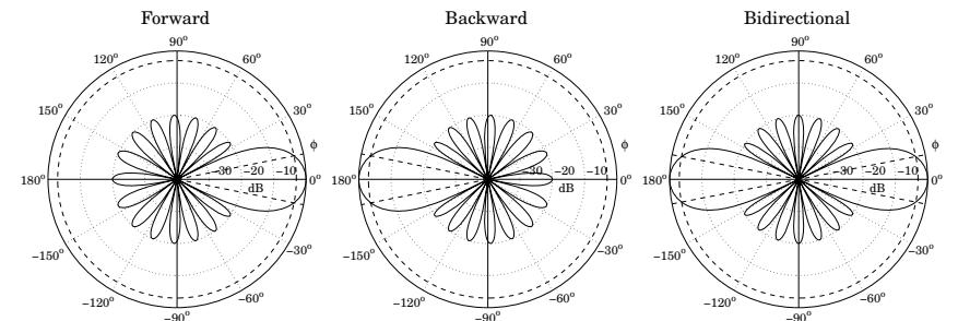
Fig. 23.9.6 Forward, backward, and bidirectional endfire designs.
