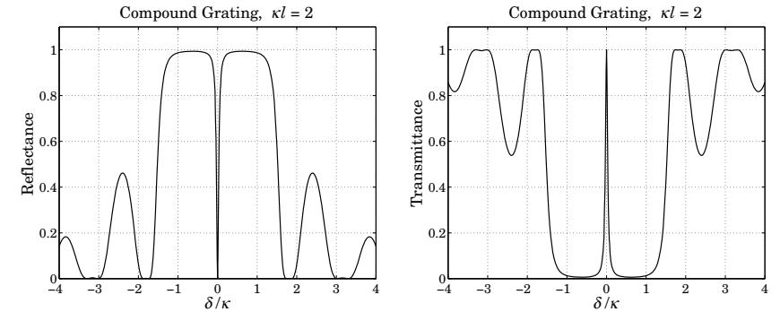
Fig. 12.5.4 Quarter-wave phase-shifted fiber Bragg grating.
