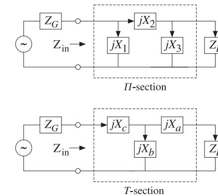
Fig. 13.12.1  $\Pi$ - and  $T$ -section matching networks.
