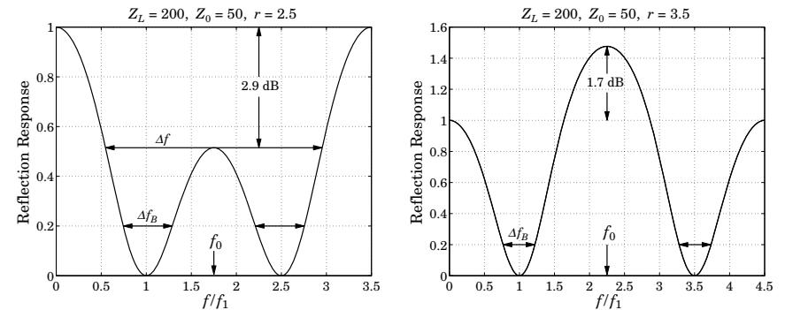
Fig. 13.4.3 Dual-band transformers at frequencies  $\{f_1, 2.5f_1\}$  and  $\{f_1, 3.5f_1\}$ .
