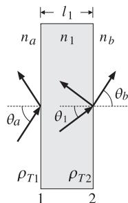
Fig. 8.3.1 Oblique incidence on single dielectric slab.
