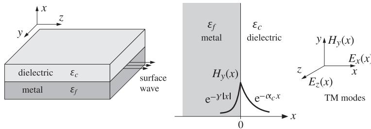
Fig. 10.2.1 Surface plasmon wave propagating along metal-dielectric interface.
