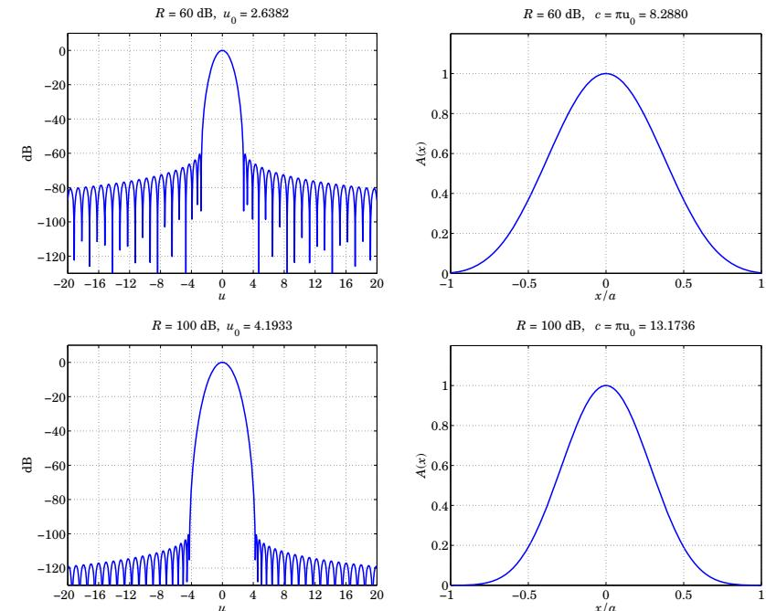
Fig. 20.13.1 Prolate window,  $|\hat{A}(k_x)|$  in dB versus  $u = ak_x/\pi$ , and  $A(x)$  versus  $x$ .
