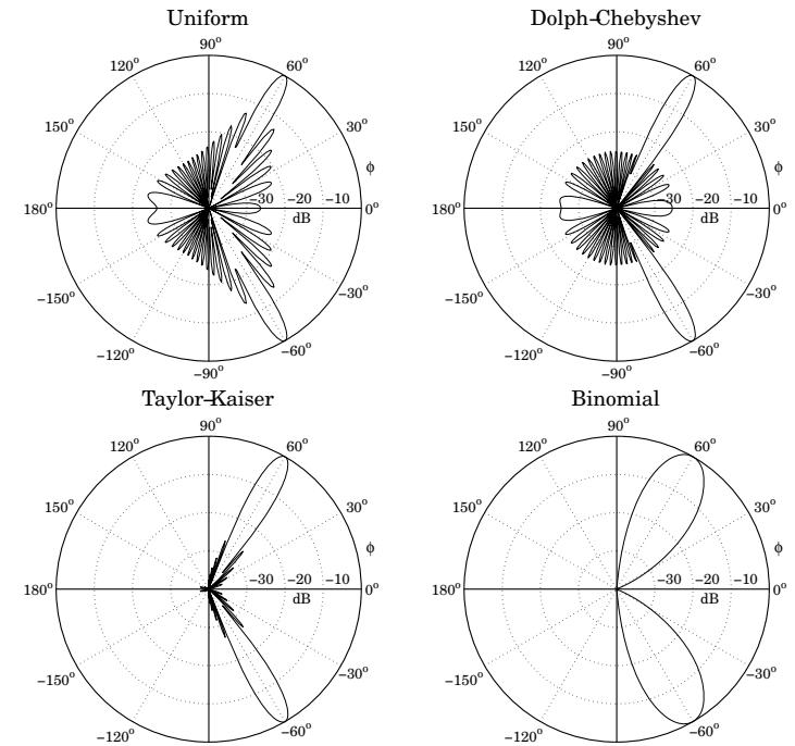
Fig. 23.7.2 Comparison of steered 21-element narrow-beam arrays.
