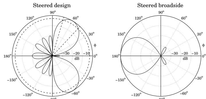
Fig. 23.9.5 Nine-element array with  $d = \lambda/4$  steered towards  $60^\circ$ .
