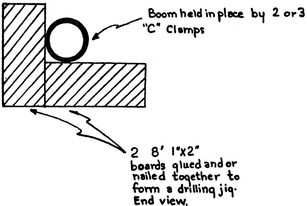
Figure 1 - Jig for drilling boom
