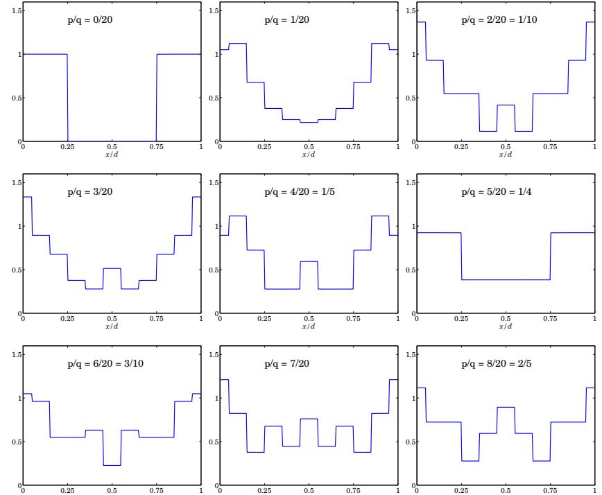
Fig. 20.2.2 Magnitude  $|E(x, z_{pq})|$  versus  $x$ , over one period,  $0 \leq x \leq d$ .
