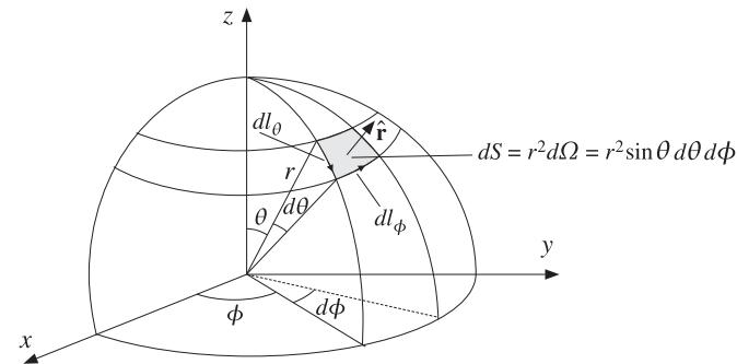
Fig. 15.8.3 Solid angle defined by angles  $\theta, \phi$ .
