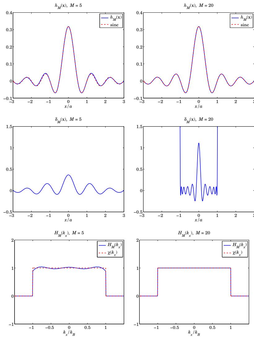
Fig. 20.22.4 Impulse response approximations, for  $M = 5$  and  $M = 20$ .
