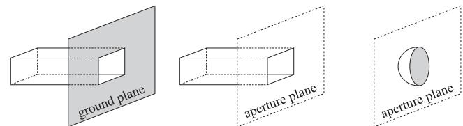
Fig. 18.1.2 Examples of aperture planes.
