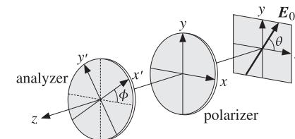
Fig. 2.14.1 Polarizer-analyzer filter combination.
