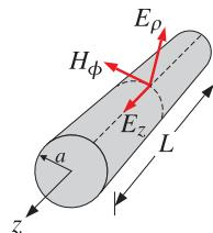
Fig. 10.16.2 Length- $L$  section of Sommerfeld wire.
