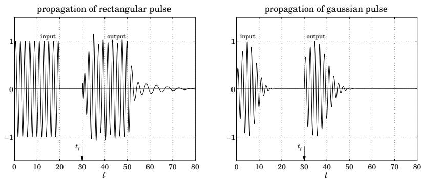
Fig. 3.4.3 Rectangular and gaussian pulse propagation.
