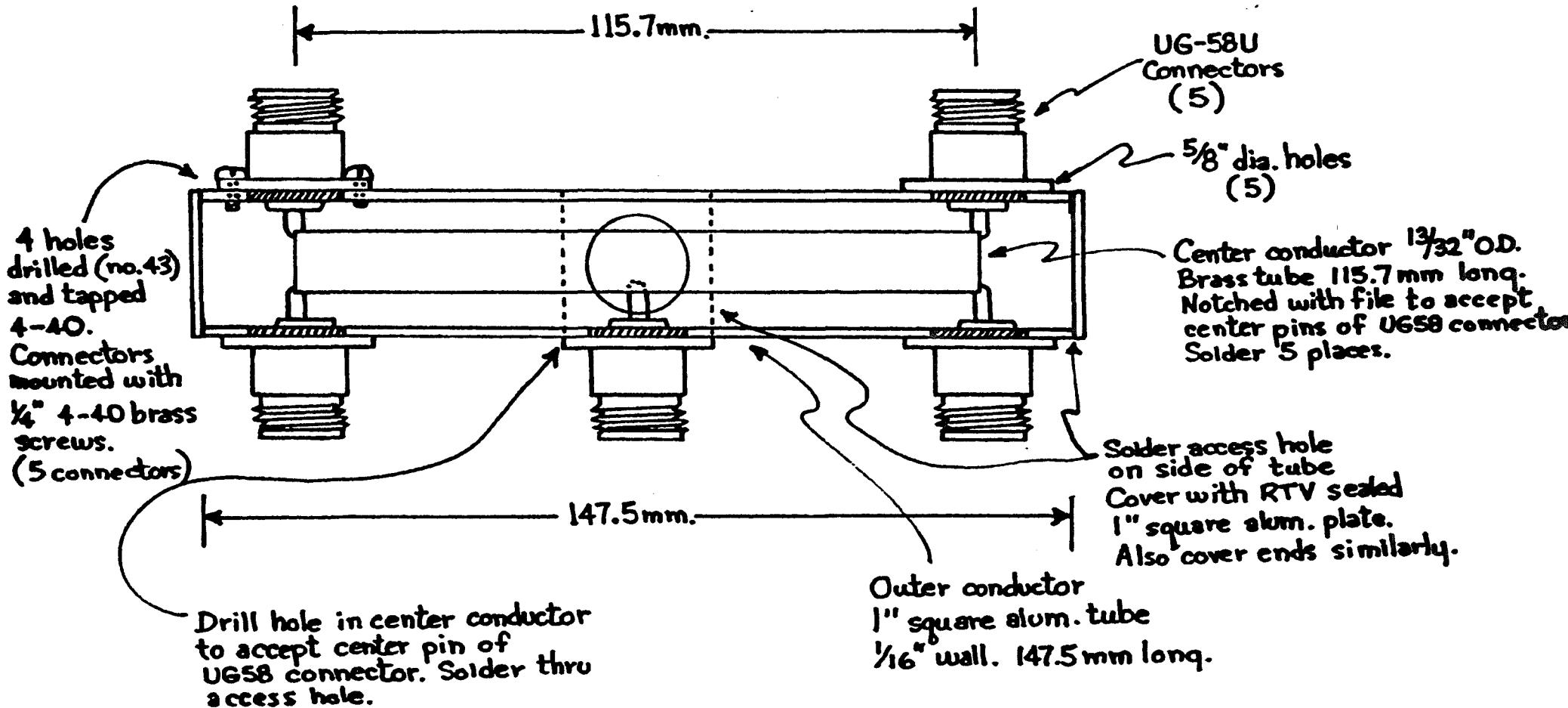
Figure 6 - 4 Port 50 Ohm Power Divider for 23 cm (1296 MHz.)
