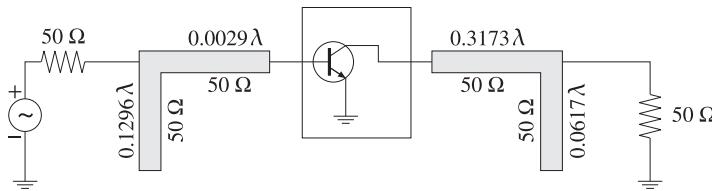
Fig. 14.10.2 Input and output stub matching networks.
