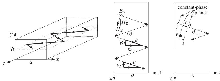
Fig. 9.9.1 Reflection model of TE<sub>10</sub> mode.
