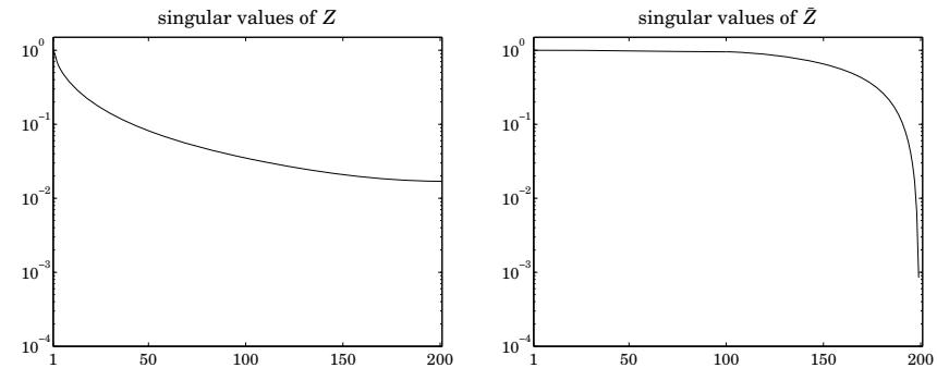
Fig. 24.14.2 Singular values of the impedance matrices  $Z$  and  $\tilde{Z}$  for  $N=2M+1=201$ .
