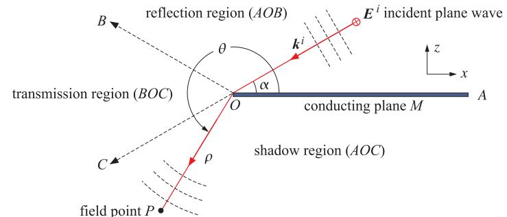
Fig. 19.10.1 Plane wave incident on conducting half-plane.
