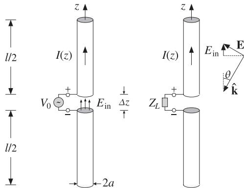
Fig. 24.2.1 External sources acting on a linear antenna.
