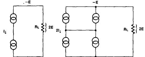
Fig. 8 Electrical Equivalent without Transformer
