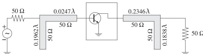
Fig. 14.8.4 Input and output stub matching networks.
