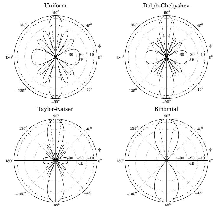
Fig. 23.7.1 Narrow beam design examples.
