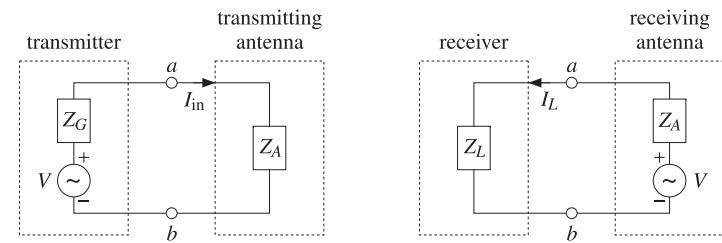
Fig. 16.4.1 Circuit equivalents of transmitting and receiving antennas.
