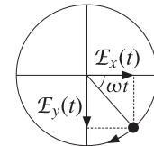
The tip of the electric field vector rotates *clockwise* on the  $xy$ -plane. Since the wave is moving forward, this will represent left-circular polarization. Fig. 2.5.1 depicts the four cases of left/right polarization with forward/backward waves.
