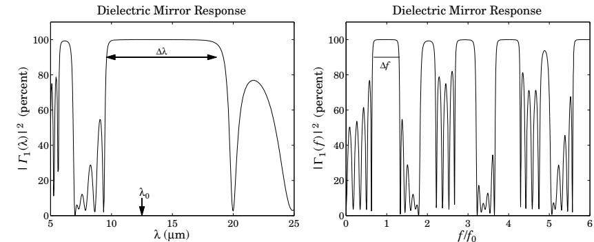
Fig. 6.3.3 Dielectric mirror with unequal optical thicknesses.
