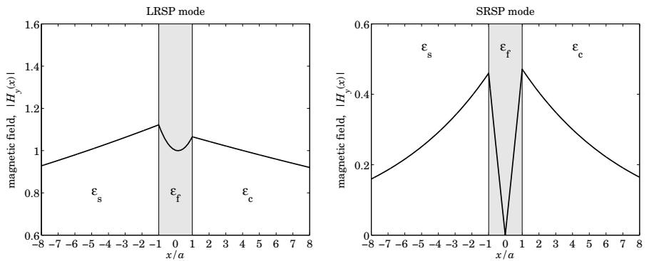
Fig. 10.13.3 Magnetic field profiles,  $2a = 20$  nm film.
