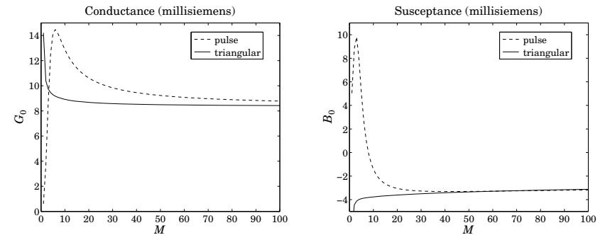
Fig. 24.11.2 Input admittance computed with pulse and triangular basis functions.
