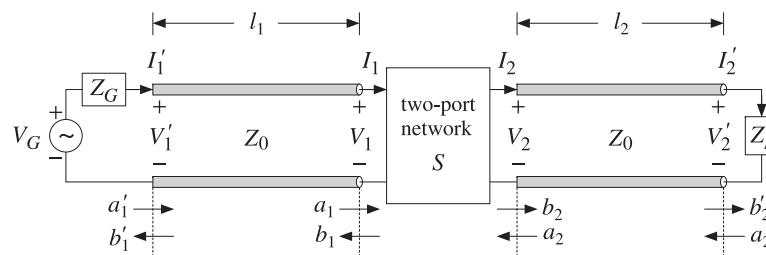
Fig. 14.1.3 Two-port network under test.
