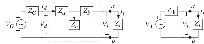
Fig. 11.11.3  $T$ -section and Thévenin equivalent circuits.
