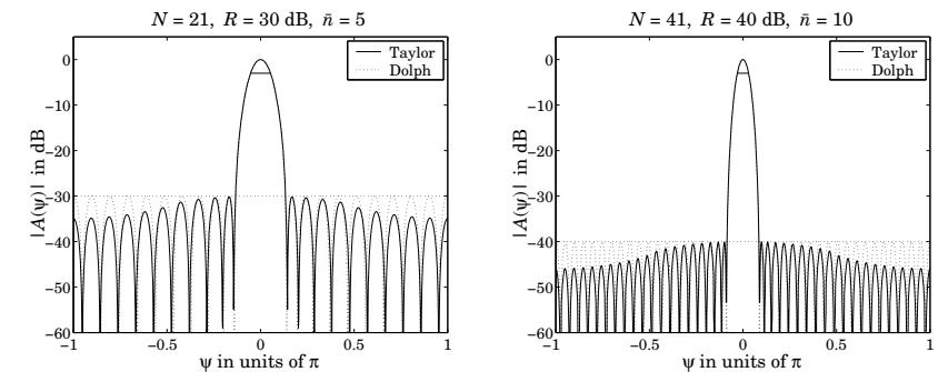
Fig. 23.12.1 Taylor  $\bar{n}$  line source array design.
