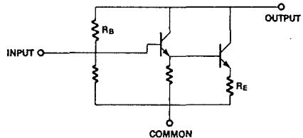
Fig. 1 RB - Shunt Feedback Resistor
