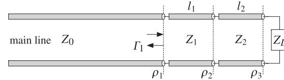
Fig. 13.4.1 Two-section dual-band Chebyshev transformer.
