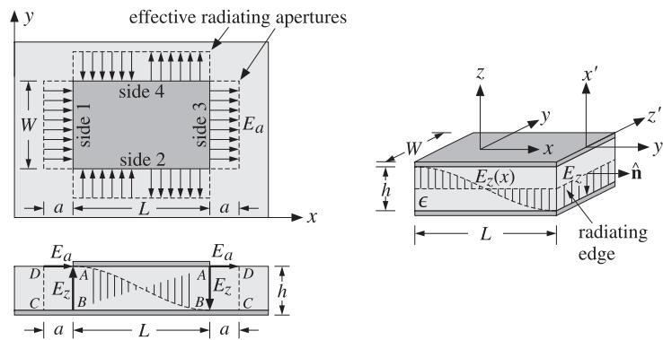
Fig. 21.6.2 Aperture models for microstrip antenna.
