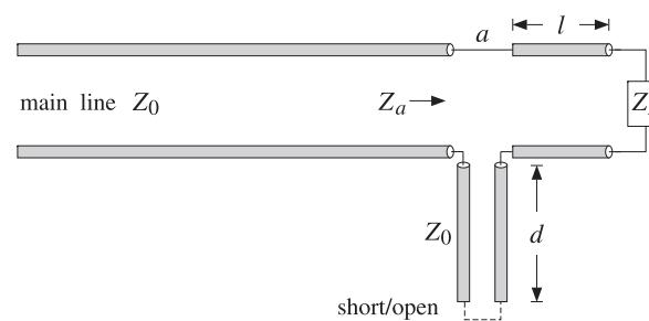
Fig. 13.8.2 Series connection of single stub tuner.
