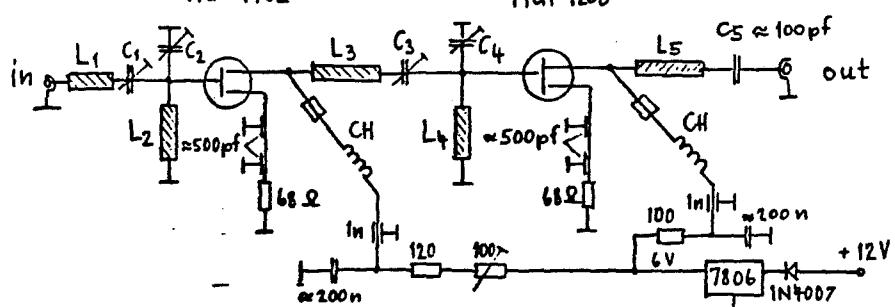
Measurements: NF < 0.6 dB, gain 35 dB
