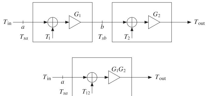
Fig. 16.8.2 Equivalent noise model of two cascaded devices.
