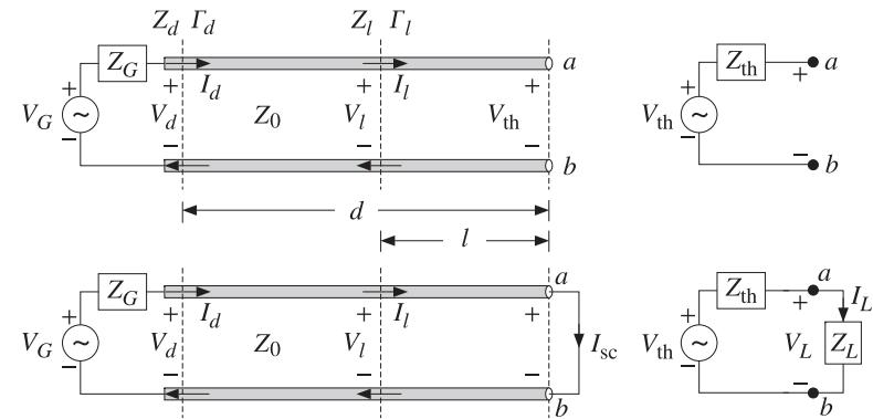
Fig. 11.11.1 Open- and short-circuited line and Thévenin-equivalent circuit.
