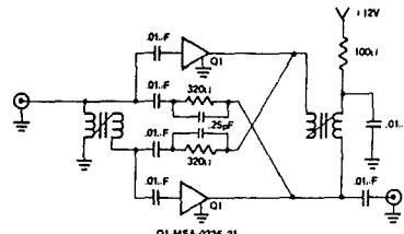
Fig. 11 Unilateraled Push-Pull Circuit
