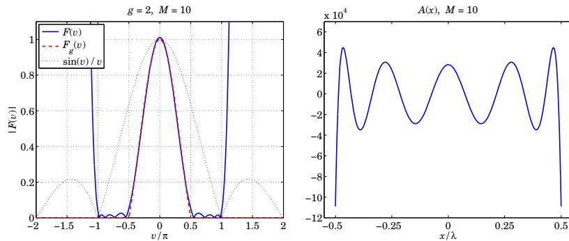
Fig. 20.22.2 Compressed sinc, with gain  $g = 2$ , and  $M = 10$ .
