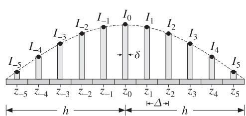
Fig. 24.9.1 Delta-function segments along an antenna, with  $N = 11, M = 5$ .
