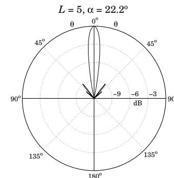
Fig. 17.7.6 Rhombic antenna gains in dB.
