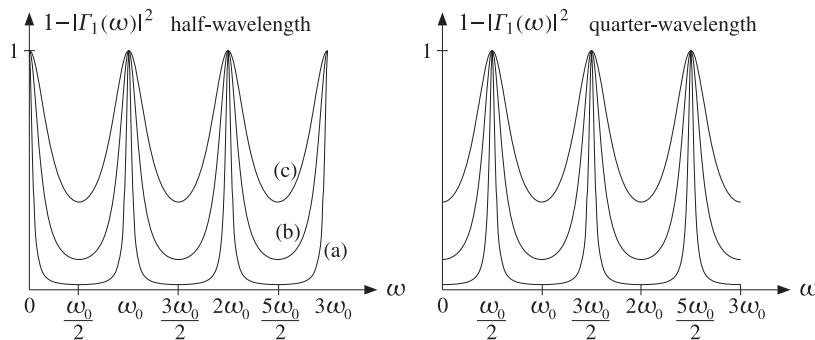
Fig. 5.5.2 Transmittance of half- and quarter-wavelength dielectric slab.
