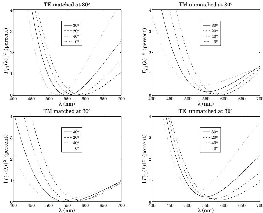
Fig. 8.7.2 Two-layer antireflection coating matched at 30 degrees.
