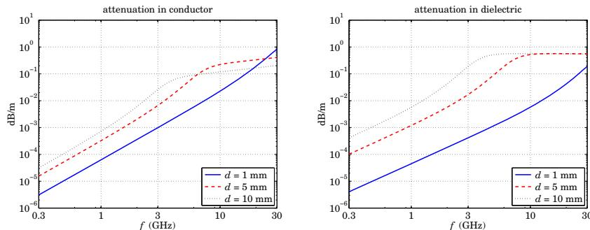
**Fig. 10.20.3** Attenuations in conductor and dielectric coating.
