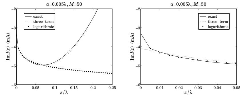
Fig. 24.10.3 Logarithmic behavior of the solution near  $z = 0$ .
