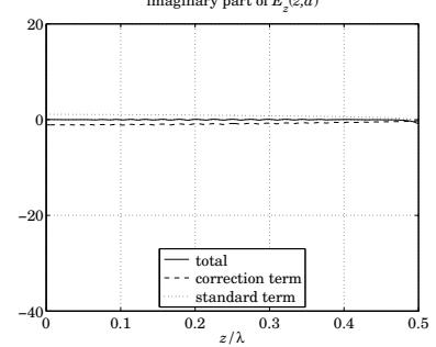
Fig. 25.2.2 Calculated near field  $E_z(z, \rho)$  for  $l = 1.0\lambda$ .
