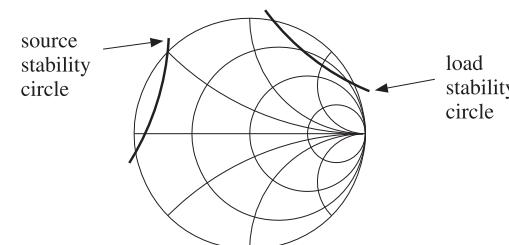
Fig. 14.5.3 Load and source stability circles at 1 GHz.
