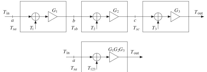
Fig. 16.8.3 Equivalent noise temperatures of three cascaded devices.
