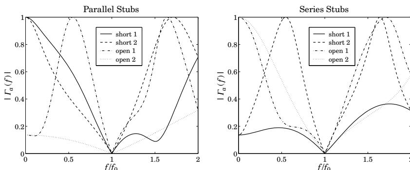
Fig. 13.8.3 Reflection response of single stub matching solutions.
