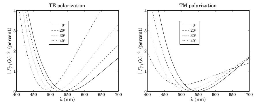
Fig. 8.7.1 Two-layer antireflection coating at oblique incidence.
