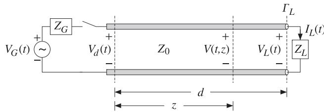
Fig. 11.15.1 Transient response of terminated line.
