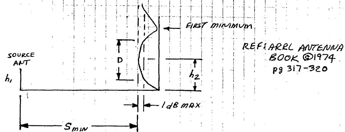
$$S_{min} = G \frac{2\lambda}{\pi^2} \text{ FOR BEST ILLUMINATION (Less than } 30^\circ \text{ phase error and } 1 \text{ dB gain variation)}$$
