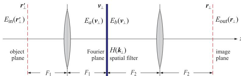
Fig. 20.11.1 4F optical processor.
