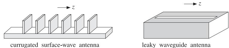
Fig. 17.6.3 Surface-wave and leaky-wave antennas.
