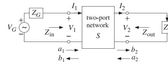
Fig. 14.1.4 Two-port network connected to generator and load.
