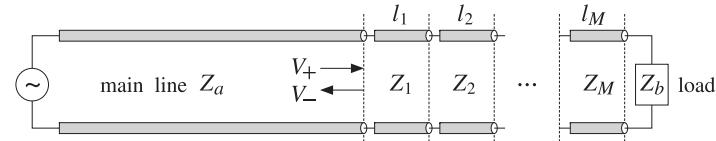
Fig. 6.7.1 Multisegment broadband termination of a transmission line.
