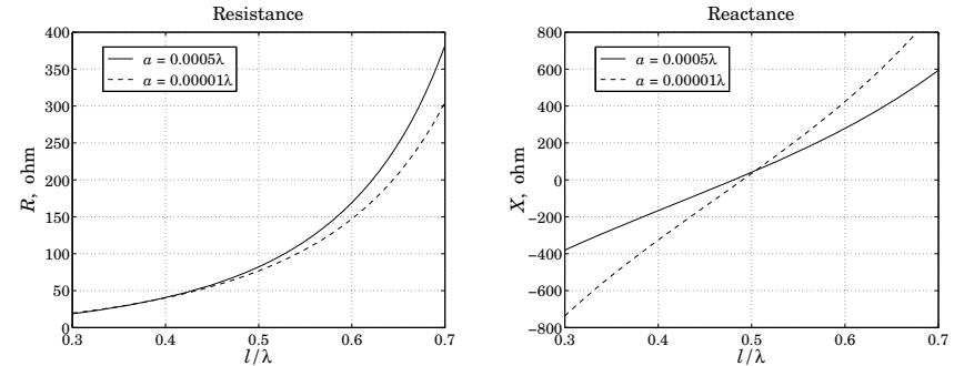
Fig. 24.10.6 Input impedance versus antenna length.
