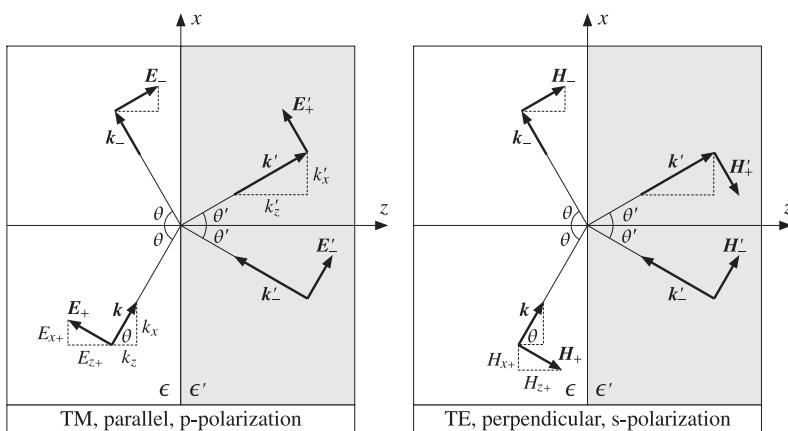
Fig. 7.1.1 Oblique incidence for TM- and TE-polarized waves.
