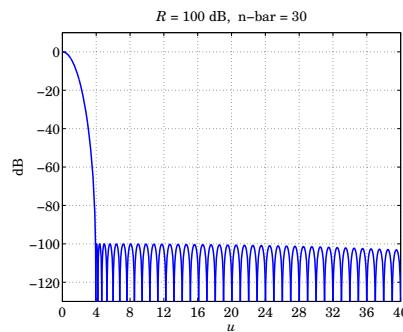
Fig. 20.15.1 Comparison of Taylor's  $n$ -bar and one-parameter windows.
