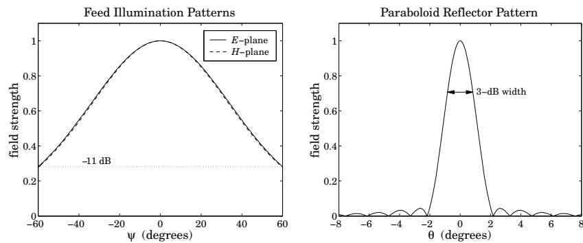
Fig. 21.10.2 Feed illumination and reflector radiation patterns.
