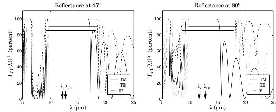
Fig. 8.8.9 Omnidirectional mirror with  $N = 8$ .
