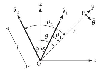
Fig. 17.7.4 Radiation vectors of traveling-wave vee antenna.
