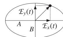
Finally, if  $A \neq B$  and  $\phi$  is arbitrary, then the major/minor axes of the ellipse (2.5.4) will be rotated relative to the  $x, y$  directions. Fig. 2.5.2 illustrates the general case.
