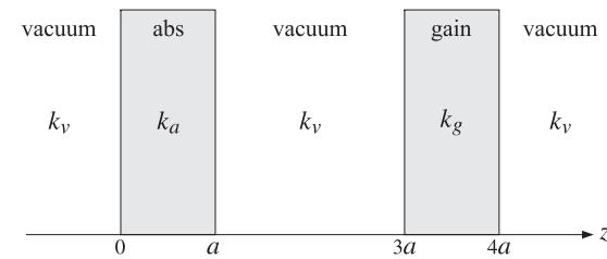
Fig. 3.9.3 Absorption and gain media separated by vacuum.
