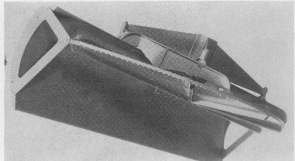
Fig. 4—Pillbox antenna feeding a cylindrical reflector.
