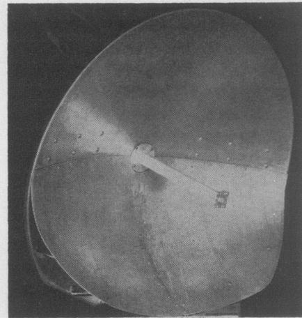
Fig. 6—Shaped-beam antenna employing a modified paraboloidal reflector.
