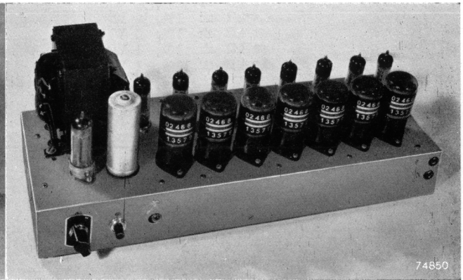
Fig. 17. Complete decade counter containing seven counter stages. The first counter tube at the left registers the millions, the second the hundred thousands, and so on. The press-button at the left serves for resetting all counter tubes simultaneously to zero. Cabinet dimensions: width 43 cm, height 17.5 cm. Depth 15.5 cm. Weight: 7.5 kg. Power consumption: 77 VA.
