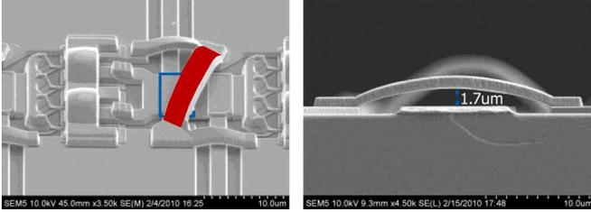
Fig. 5. SEMs of 670-GHz SSPA interstage matching network (left) and airbridge detail (right).
