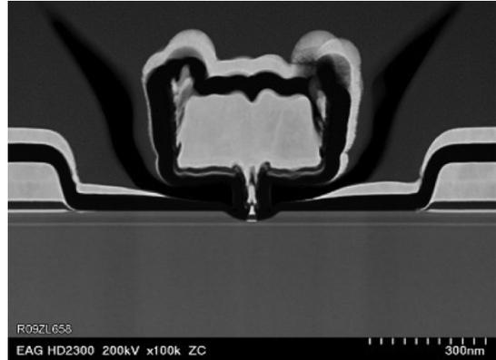
Fig. 1. Scanning Electron Tunneling (SEM) image of 30-nm InP HEMT gate.
