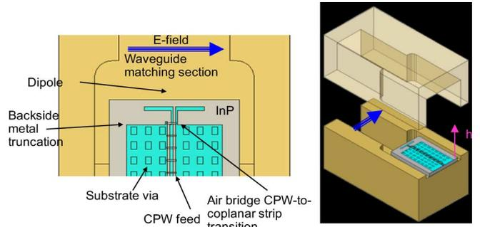
Fig. 6. Schematic of integrated coplanar waveguide to waveguide transition.
