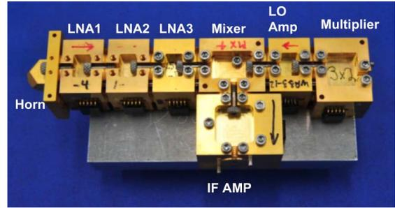
Fig. 18. A 670-GHz receiver with all functions realized in InP HEMT.
