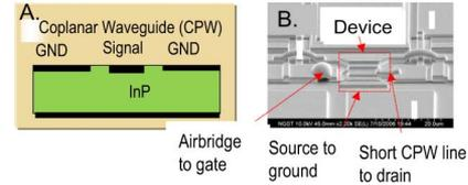
Fig. 3. Details of passive technology for Terahertz InP HEMT process.
