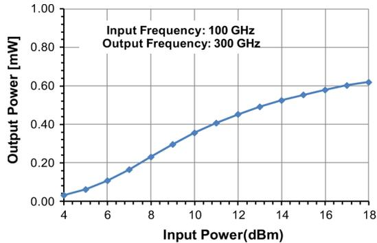
Fig. 17. Measured input power versus output power of the frequency tripler.
