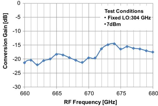
Fig. 15. Measured down conversion loss of sub-harmonic mixer.
