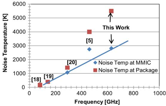
Fig. 20. Northrop Grumman InP HEMT noise temperature trend chart.
