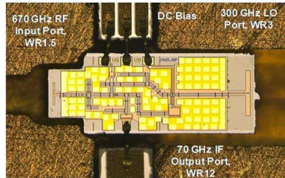
Fig. 14. Microphotograph of InP HEMT sub-harmonic down converting mixer in waveguide fixture.
