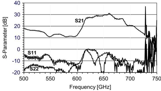
Fig. 11. Measured on-wafer S-Parameters of 10-stage LNA.
