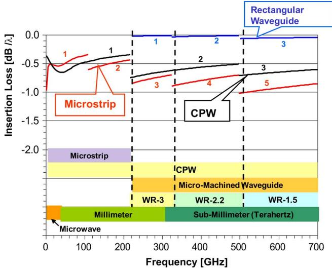
Fig. 4. Loss per wavelength for various kinds of transmission lines and waveguides as a function of frequency.
