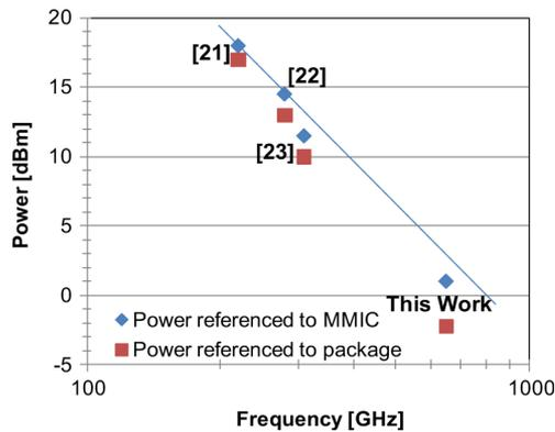
Fig. 21. Plot of measured output power versus frequency for 30- and 35-nm InP HEMT.
