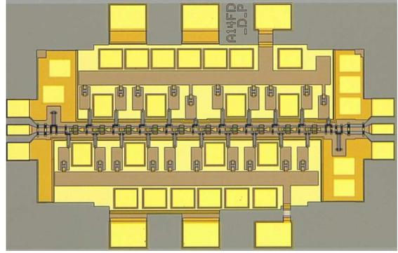
Fig. 10. Microphotograph of 10-Stage 670-GHz low noise amplifier.
