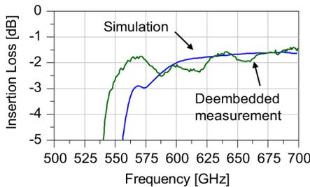
Fig. 9. De-embedded insertion loss of a single transition.
