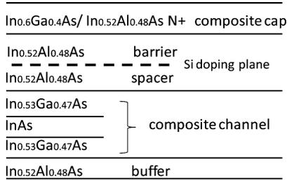
Fig. 2. Layer profile of the epi wafers.
