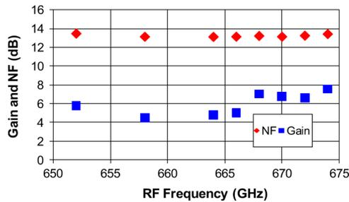
Fig. 12. Measured noise performance of packaged 5-stage low noise amplifier.
