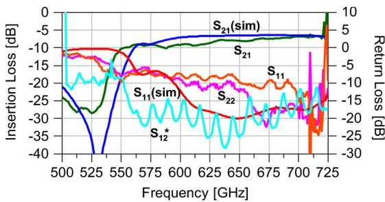
Fig. 8. Measured performance of WR1.5 package with CPW through line.
