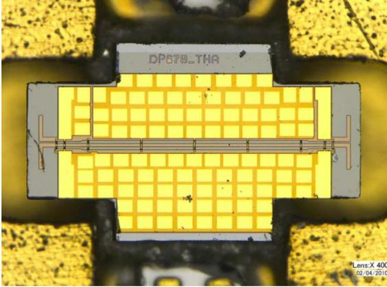
Fig. 7. Microphotograph of CPW through line with WR1.5 waveguide transitions at either end.
