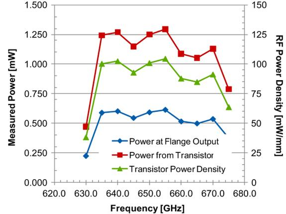
Fig. 13. Measured output power from 5-stage LNA.
