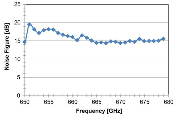
Fig. 19. Measured noise figure of receiver.
