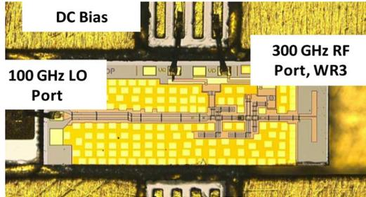
Fig. 16. Microphotograph of InP HEMT frequency tripler in waveguide fixture.
