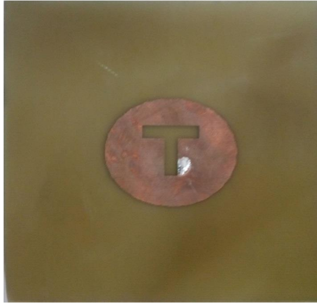
Figure 12: Top view of proposed antenna
