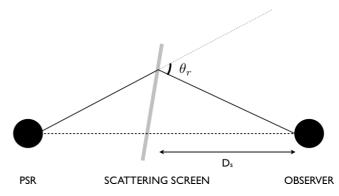
**Fig. 8.** A gradient in the electron density perpendicular to the line-of-sight causes rays to be bent. The size of the angle which the rays are bent through depends on the frequency of the radiation. Low frequencies (dark line) are bent through a larger angle and so must travel along a longer path to reach the observer, delaying them with respect to higher frequencies (dashed line).
