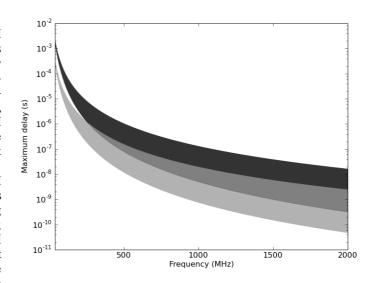
**Fig. 6.** These curves show the upper limits on the size of delays from second-order ISM effects extrapolated up to higher frequencies. The dark grey area is for PSR B0809+74, which had the largest RMS residuals in our timing fits; the light grey area is for PSR B1919+21, which had the smallest RMS residuals. They are scaled with  $v^{-3}$  and  $v^{-4}$  which are the lower and upper bounds for scaling of the second-order ISM effects.
