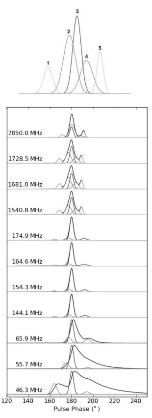
**Fig. 9.** The model of PSR B0329+54 used for the dynamic template. The pulsar is modelled using five Gaussian components (plotted with grey lines). At low frequencies the model is convolved with an exponential function to account for the effects of scatter broadening. The final model (including the scatter broadening) is plotted in black.
