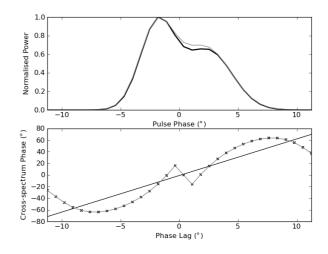
**Fig. 2.** Errors in timing PSR B1919+21. The top panel shows the HBA template (black line) and the 145 MHz data (grey line). The bottom panel shows the cross-spectrum phase of the template and the profile and a straight line fit to the data (solid line). The subtle difference between the shape of the pulse profile and the template causes a gradient in the cross-correlation phase shifting the apparent TOA.
