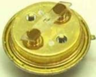
10 MHz, 3rd Overtone SC (Stress-Free) Cut Crystal
