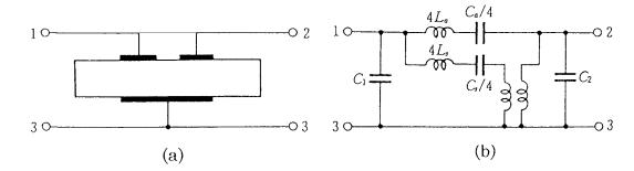
Fig. 6. The symbolic circuit of a crystal filter using multi-energy trapping vibration modes and (b) the equivalent circuit.
