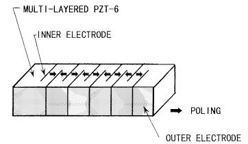
Fig. 12. The physical configuration of a 450-kHz ceramic resonator using multi-layered PZT ceramics.
