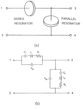
Fig. 2. (a) An L-section of a ladder-type ceramic filter with ceramic resonators in the series and parallel branches and (b) the equivalent circuit.
