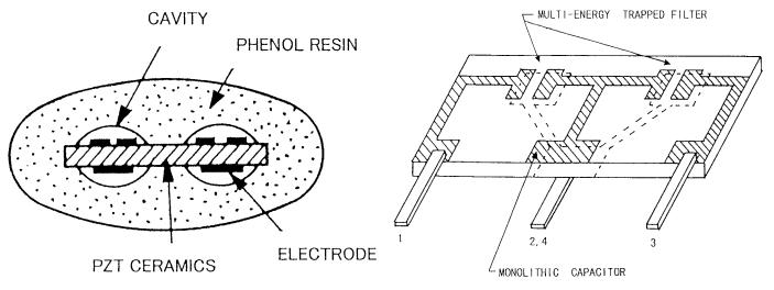
Fig. 7. The package of a 10.7-MHz ceramic filter.
