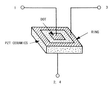
Fig. 4. The physical configuration of a 455-kHz ceramic filter.
