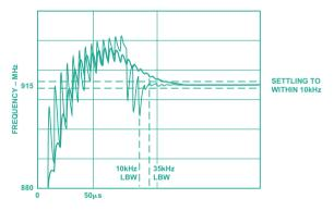
Figure 5. Loop bandwidth has a significant effect on the lock time. The wider the loop bandwidth, the faster the lock time, but also the greater the level of spurious components. Lock time to 1 kHz is 142  $\mu$ s with a 35-kHz LBW—and 248  $\mu$ s with a 10-kHz LBW.
