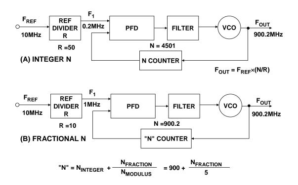
Figure 7: Integer-N Compared to Fractional-N Synthesizer
