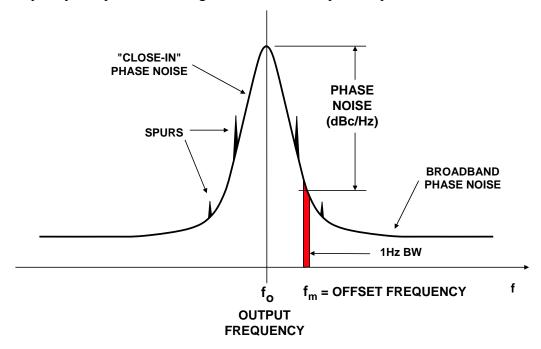
Figure 5: Oscillator Phase Noise and Spurs
