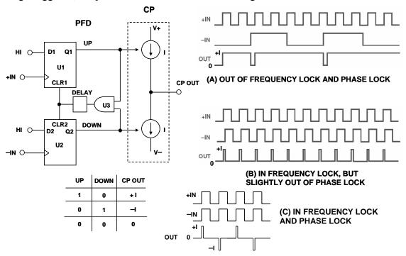
Figure 2: Phase/Frequency Detector (PFD) Driving Charge Pump (CP)
