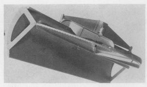
Fig. 4—Pillbox antenna feeding a cylindrical reflector.
