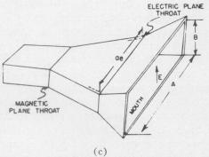
Fig. 1—Horn-feed types. (a) Electric-plane horn. (b) Magnetic-plane horn. (c) Compound horn.
