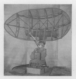
Fig. 2-Antenna with asymmetrically cut reflector.
