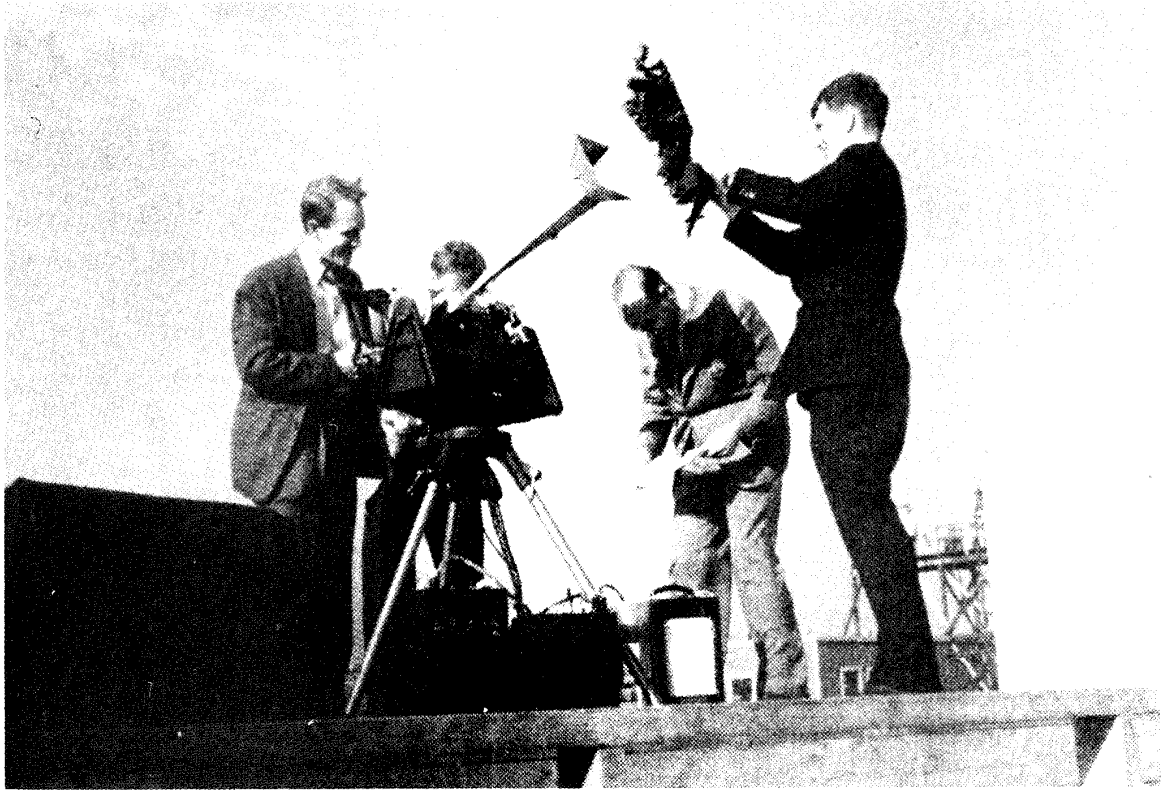
Fig. 1. Dicke shakes the "Shaggy Dog" calibrator in front of the 1 cm radiometer used to measure atmospheric absorption. Also in the picture: E. Beringer, R. Kyhl and A. Vane.
