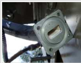
Flexible waveguide from a J-Band radar
