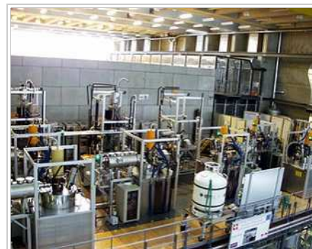
High power 84 - 118 GHz gyrotron tubes for plasma heating in the TCV tokamak fusion reactor, Switzerland. The colored cylinders are the tops of the gyrotron tubes.
