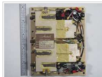
Figure 6: 8–12 GHz tunnel diode amplifier, circa 1970
