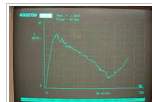
I-V curve of 10mA germanium tunnel diode, taken on a Tektronix model 571 curve tracer.
