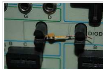
10mA germanium tunnel diode mounted in test fixture of Tektronix 571 curve tracer
