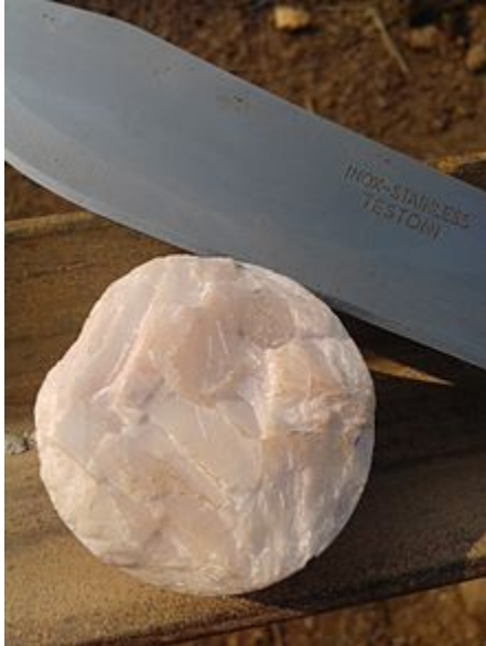
Quartz mineral embedded in limestone (top right of the sample), easily identifiable by its hexagonal form. It cannot be scratched by steel (see Mohs scale).
