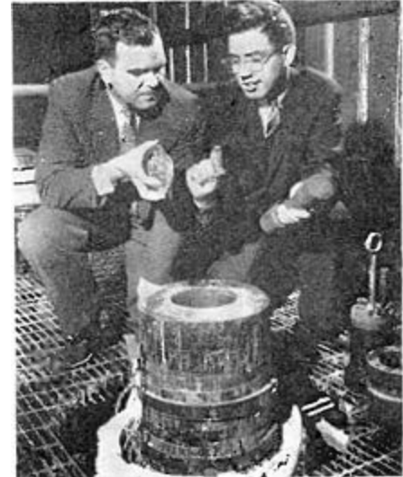
Synthetic quartz crystals produced in the autoclave shown in Western Electric's pilot hydrothermal quartz plant in 1959
