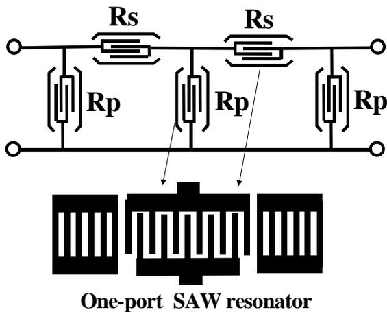
(c) Ladder type SAW filter design
