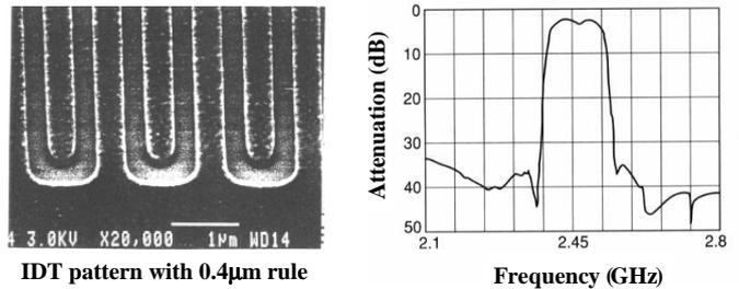
Fig.8 IDT pattern and 2.4GHz SAW filter
