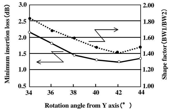
**Fig.6 Experimental results for optimizing the cut angle**
