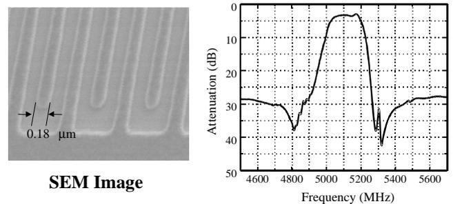
Fig.9 IDT pattern and 5 GHz SAW filter
