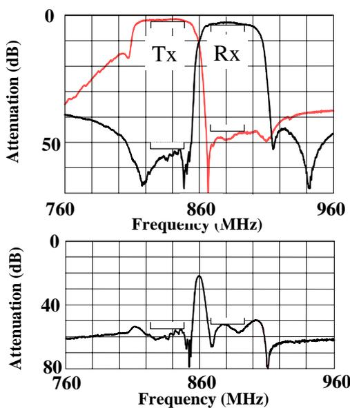
Fig.15  $S_{21}$  characteristics for AMPS duplexer
