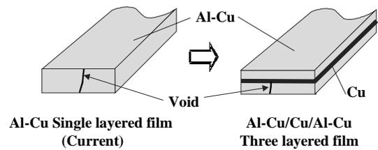
Fig.11 The structure of three layered film.
