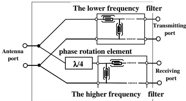
Fig.13 The structure of antenna duplexer
