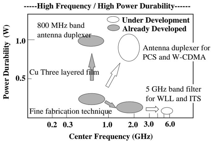
Fig.17 Trend of RF SAW filter development
