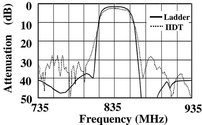
Fig.2 A comparison between ladder and IIDT
