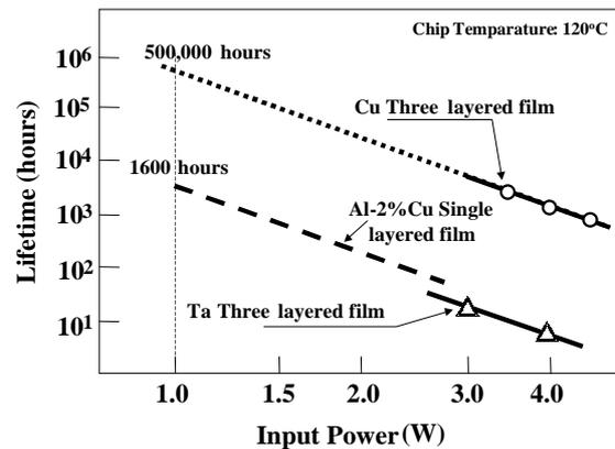
Fig.12 The lifetime vs. input power.
