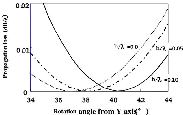
**Fig.5 The propagation loss dependency on the rotation angle from Y axis in LiTaO<sub>3</sub>**
