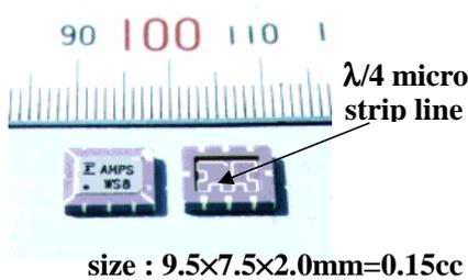
Fig.14 The photograph of SAW duplexer
