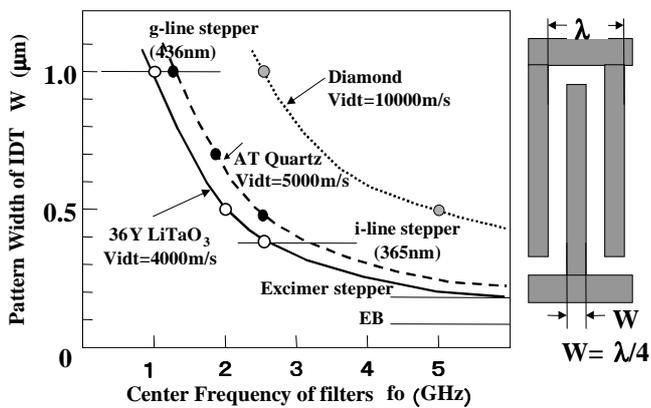
Fig.7 The frequency of filter vs. pattern width
