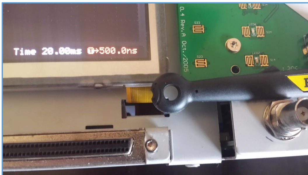
Figure 7-5: Measuring a display ribbon cable for emissions using an H-field probe.
