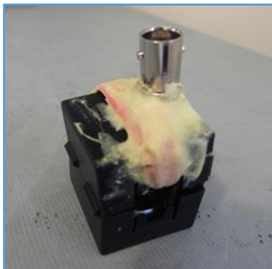
Figure 7-13: Hand-made current probe.
