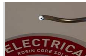
Electrical solder with an integrated rosin core, visible as a dark spot in the cut end of the solder wire.
