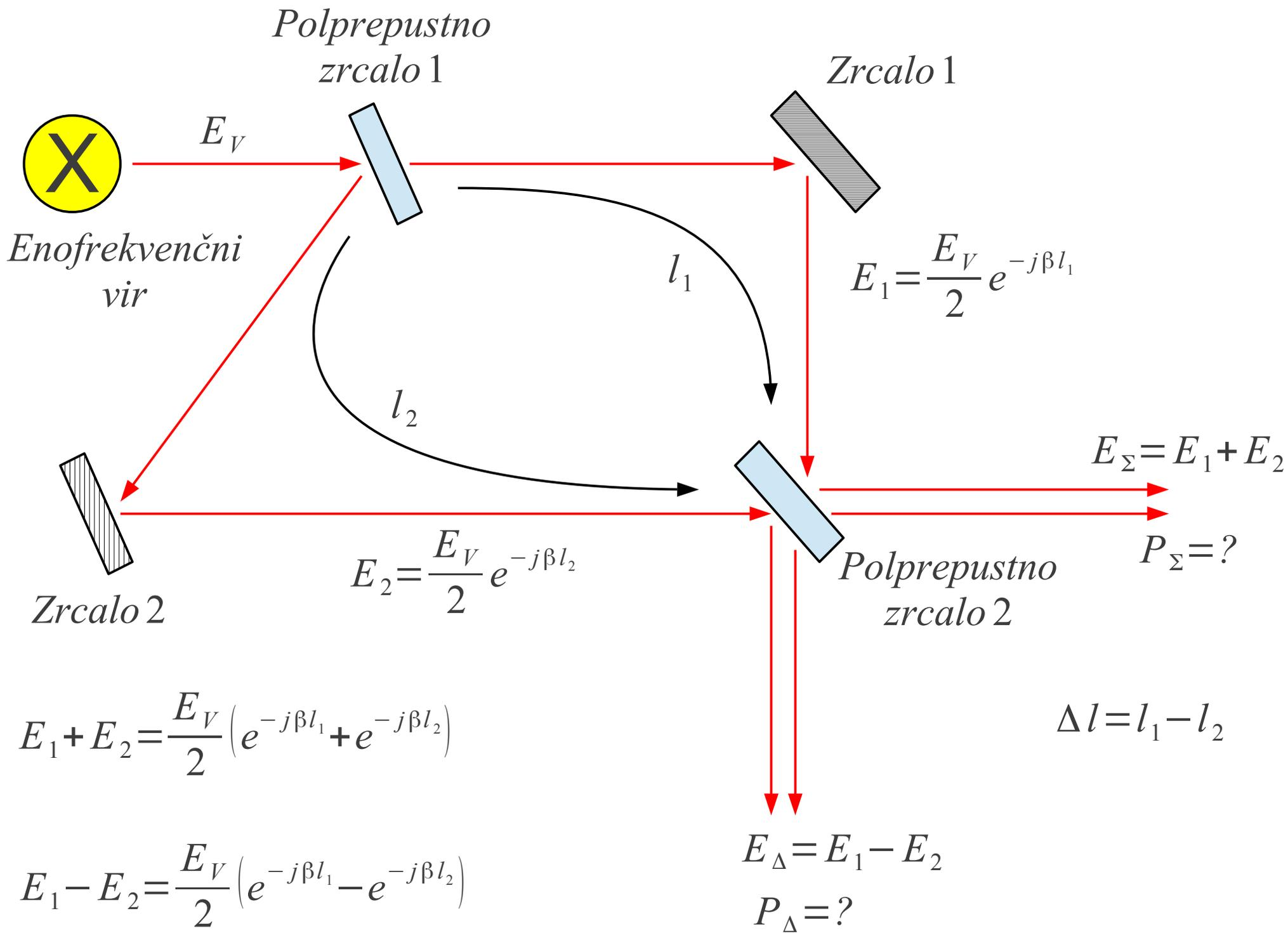
$$E_{\Sigma} = E_1 + E_2 = \frac{E_V}{2} (e^{-j\beta l_1} + e^{-j\beta l_2}) = E_V e^{-j\beta \frac{l_1+l_2}{2}} \cos \beta \frac{\Delta l}{2} \quad P = \alpha |E|^2$$
